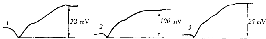
Fig. 5. Piezoelectric effect manifesting itself in the composites IKVOBAN-U2 before carrying out the implantation test (1), after removal from the organism of an animal (12 months) (2) and subsequent drying (3).
